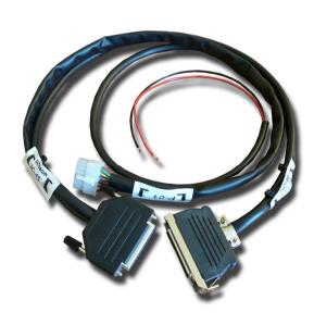
IC-15 intercom with the AR 4201 transceiver. In the offer, also installations for different transceiver model are to be found. The complete offer in the Web site at: www.olk.com.pl With aid of this installation, the task is limited to interconnection between intercom and transceiver, as well as connection to power source. Attachment of headphone sockets is best achieved with the connector card, specified in the next page.
