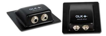
The presented case allows to install the headset sockets so that the jacks are parallel to cockpit side-board. Particularly helpful in aircraft, where the sockets are installed close to seats, and the adjustable seat is passing the headset jacks. Installation of headset jacks in a case prevents breaking the jacks away.
