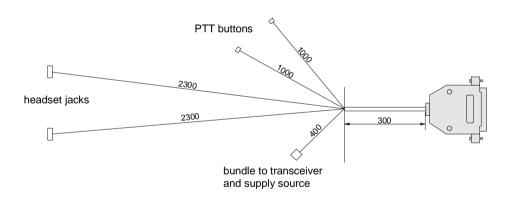
Length of wire bundles allows for installation of Intercom in almost every light aircraft.
