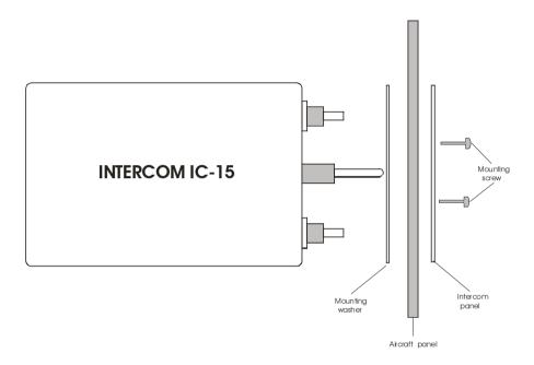
The mounting washers are used to support the intercom block so, that the block rests with all area of its front face against mounting panel. If the aircraft mounting panel is thick enough, to allow the intercom front face to rest on it, there is no need for spacing washers. With correct installation, the screws will not tend to "draw in" the intercom panel.
